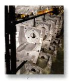
Many of the coating lines were originally designed to coat one substrate – often times cast or cold rolled steel. These coating lines are now being tasked with coating multiple metals, sometimes side by side on the same rack.
