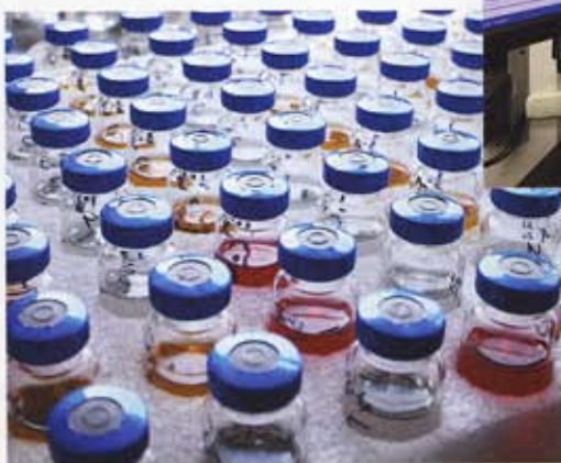
⊕ Lab analysis (above) monitors water used in fracturing. Bacteria monitoring (right) optimizes biocide selection and reduces formation fouling.
